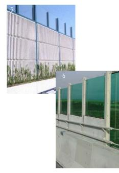
IMAGES 5-6 DISPLAY THE EFFECTIVE USE OF TRANSPARENCY TO REDUCE THE VISUAL IMPACT OF THE BARRIER
